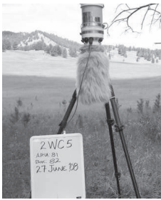
An recording unit used in the Black Hills. The fur shields the microphone from wind noise.
